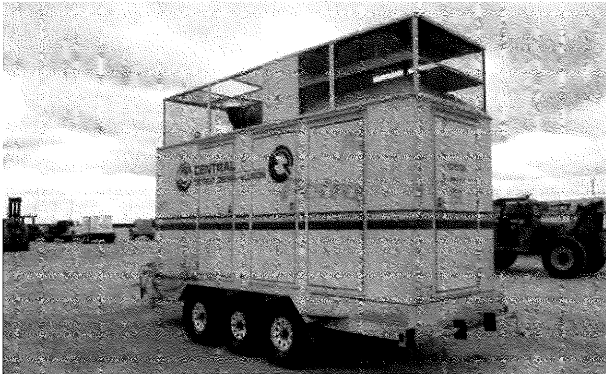
Photo of a portable Detroit Diesel Spectrum 350. From an observation stand point, it may require a minimum of a \frac{3}{4} to a 1 ton truck to pull it. The District service vehicles (trucks) are \frac{1}{2} tons.
